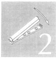
Press the body onto the back of the base plate until fixed.
