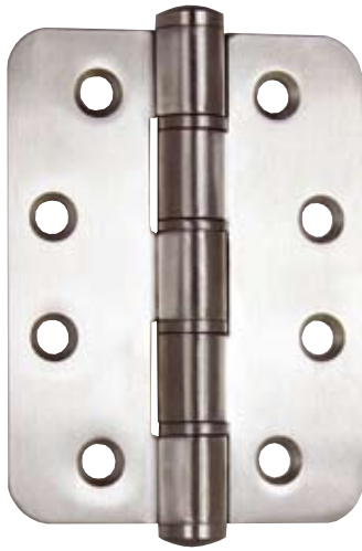
BUTT HINGE "ROUND" 102 X 76 X 3 MM Item No. 15.20.116 Incl. CSK SS-304 screws Ø5 x 30 mm
